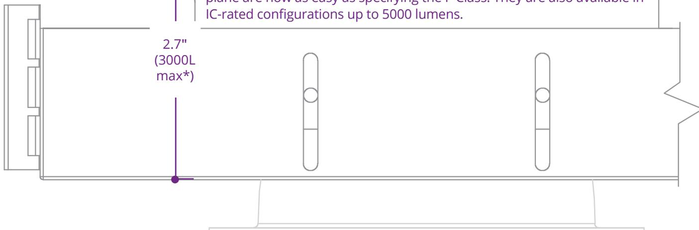
\* Fixture depth = 3" at 4000L and 5000L outputs
